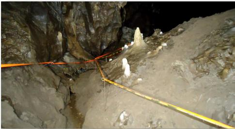
The biggest difficulty was making the pins secure as they usually grounded on rock before any depth had been attained, a situation that had proved problematic during the original taping exercise. We overcame the problem by drilling small holes to a suitable depth. We lost count of how many pins we used. Out of the original 40 or so many were shortened to make two or three out of one. Bending the end of the new short pins was achieved by drilling a hole in a stone
